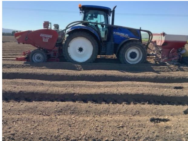
Front hopper (fertiliser) & rear hopper (potatoes).
