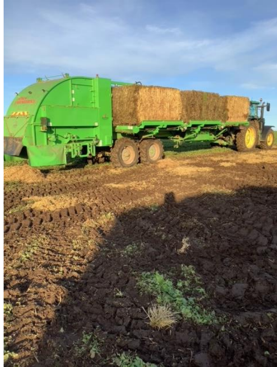
1. Machine almost empty lowering its "wings" for more bales. 2. Loading bales.
